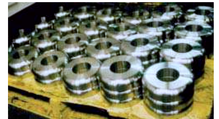
Rollers for sheet folding in Z155CDV12 hardened 58/60 HRC
