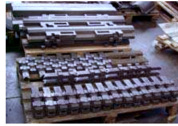
DIFFERENT TYPES OF STRIPPING PLATES FOR WIRE MILLS
