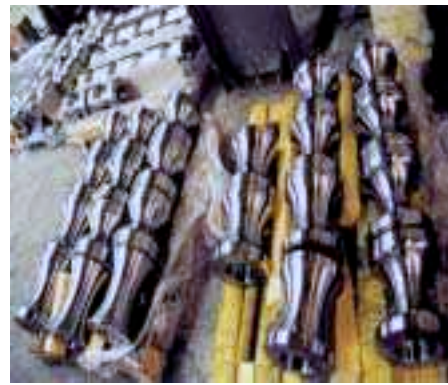
DIFFERENT KIND OF GROOVED ROLLS FOR ROLLING MILLS : Train for wire & bar
