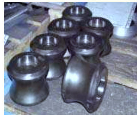
DIFFERENT KIND OF ROLLS FOR ROLLING MILLS: Guiding, twisting and straightening rolls
