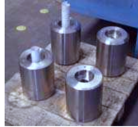
DIFFERENT KIND OF ROLLS FOR ROLLING MILLS: Guiding, twisting and straightening rolls
