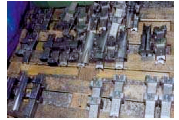
DIFFERENT TYPES OF STRIPPING PLATES FOR WIRE MILLS
