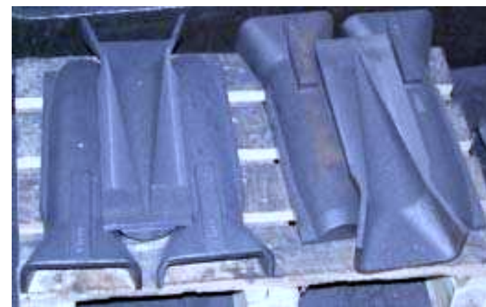
ROUGH HALF-GUIDES BEFORE MACHINING
