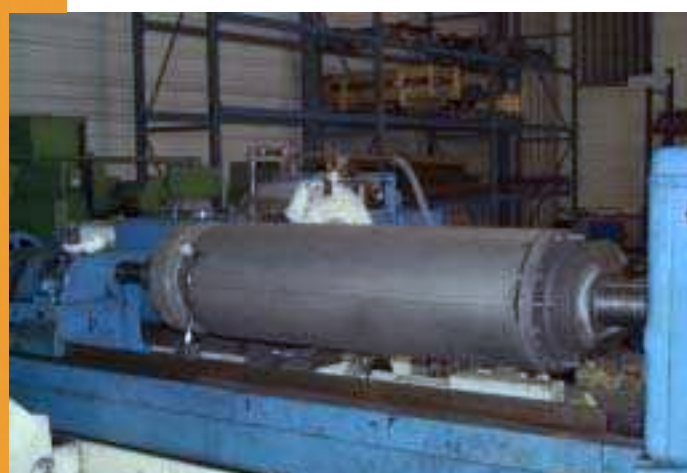
SHOT-BLASTED MANDREL DURING GRINDING
